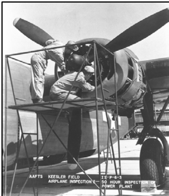
Students perform a 50-hour inspection of the power plant of a B-24 at Keesler Field.
