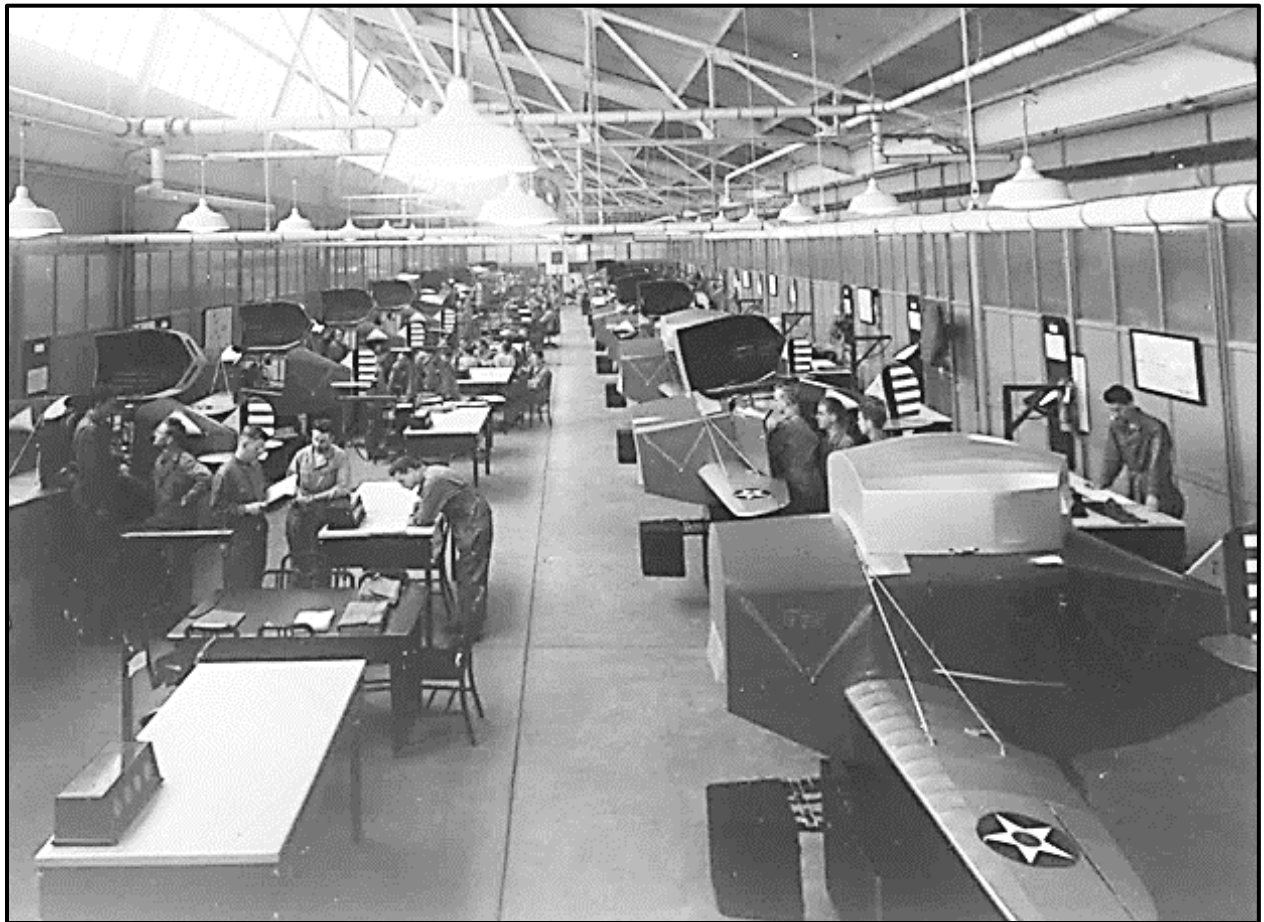
Rows of link trainers fill this classroom at Chanute Field, Illinois. Air Training Command used this trainers to teach operator and maintenance technicians.
