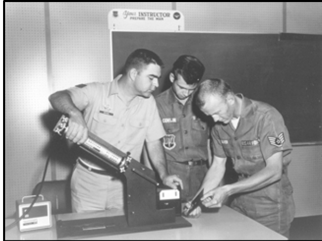
An instructor shows students a laser photo reconnaissance system and how it polarized light with a laser light source.
