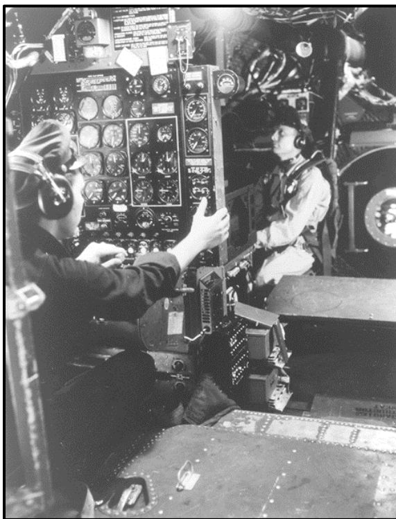
The flight engineer in a B-29 takes readings in preparation for takeoff.
