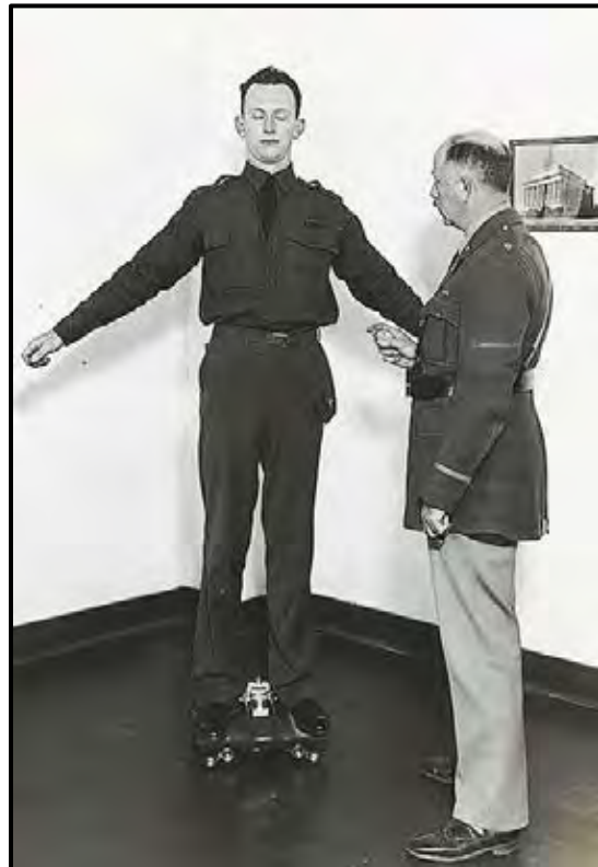
In the 1930s, the School of Aviation Medicine used the Wobblemeter as a screening device to check balance and orientation abilities of flying cadets.
