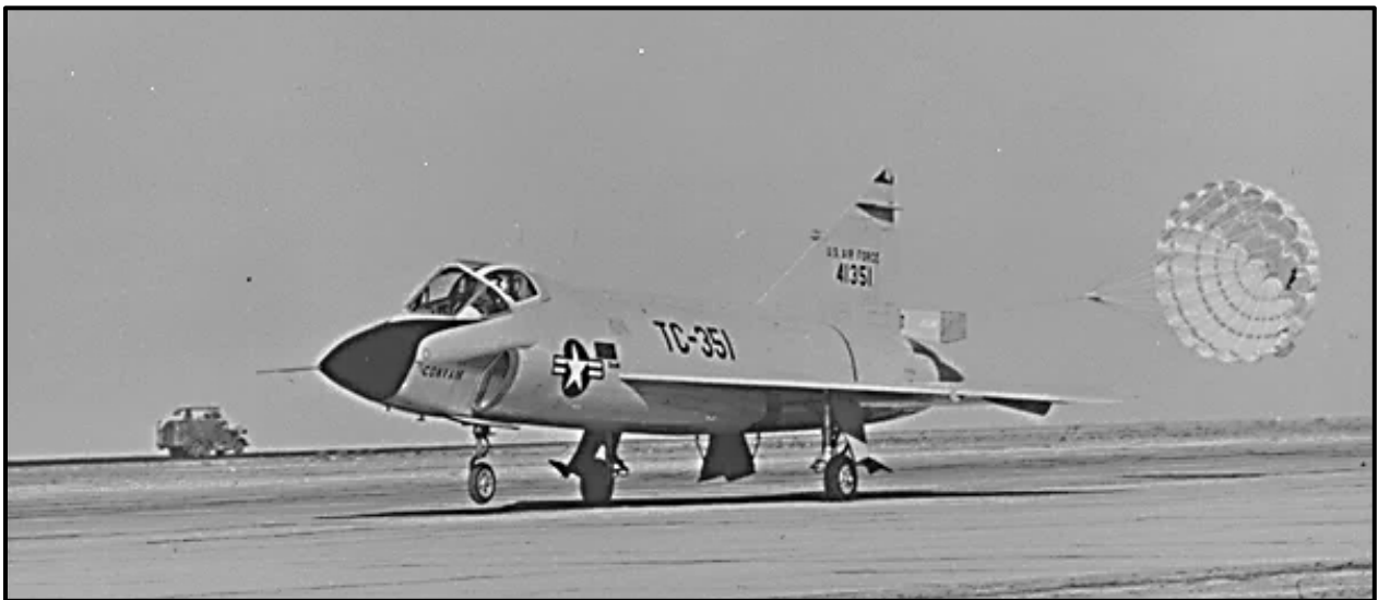
A Convair TF-102A Delta Dagger trainer lands at Edwards AFB, California, with a drag chute. This trainer from Perrin AFB, Texas, was similar to the F-102A but had a wider front fuselage seating two side-by-side.
